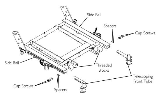
FIGURE 6.7 Adjusting/Replacing Telescoping Front Rigging Support
